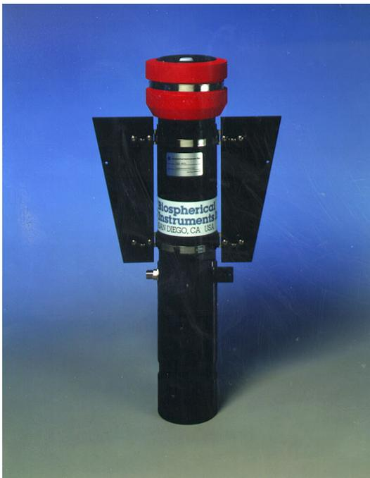
The PRR-800 is intended to be lowered from a vessel supported by its own cable. The instrument can be used in traditional vertical profiling or, when fitted with an optional free-fall collar (shown above), in free-descent mode. The free-fall system allows the researcher to “kite” the instrument away from the vessel, thereby avoiding problems caused by ship shadow.
