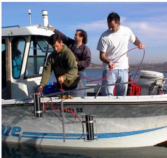
The PRR-800 is also available in an optional split configuration for use in turbid waters.
