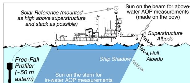
**Fig. 66.** A schematic representation of the platform perturbations associated with a ship and deployment locations for AOP measurements.
