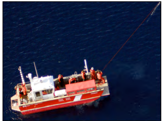
Fig. 70. The EM25 telescoping mast extended on the small boat (port side, stern) launched from the CCGS Amundsen during C-OPS deployment operations. Note the red cable extending from the port bow and the white streak (top right corner) from the cable being hauled in.
