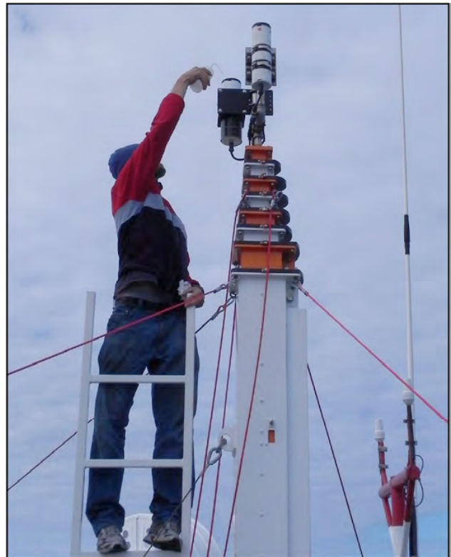
Fig. 72. The FM60 telescoping mast collapsed, with the solar references being cleaned prior to the recording of dark measurements (caps on).
