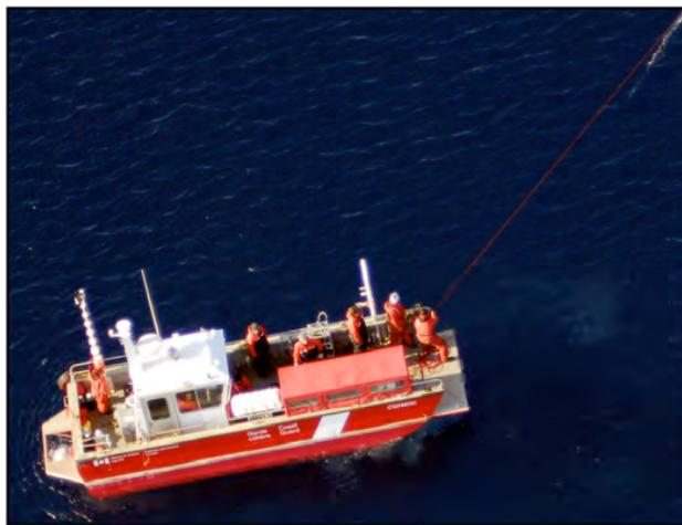
**Fig. 70.** The EM25 telescoping mast extended on the small boat (port side, stern) launched from the CCGS *Amundsen* during C-OPS deployment operations. Note the red cable extending from the port bow and the white streak (top right corner) from the cable being hauled in.
