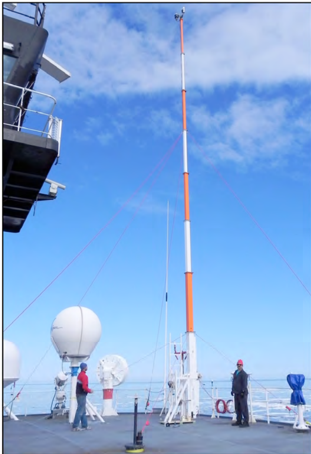
Fig. 71. The FM60 telescoping mast mounted on top of the USCGC Healy with Kevlar guy lines attached.
