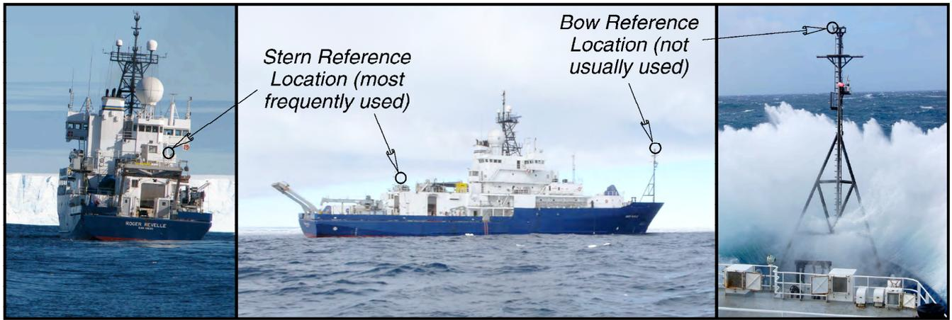
**Fig. 67.** Stern (left), side (middle) and bow (right) views of the R/V *Roger Revelle* showing a typical location for a solar reference towards the stern and the preferred (but more difficult) location on the bow. Although not as high as the tallest mast on the ship, the latter is substantially above and far away from the most substantial part of the superstructure, and provides significant shelter for the reference even in high sea states.
