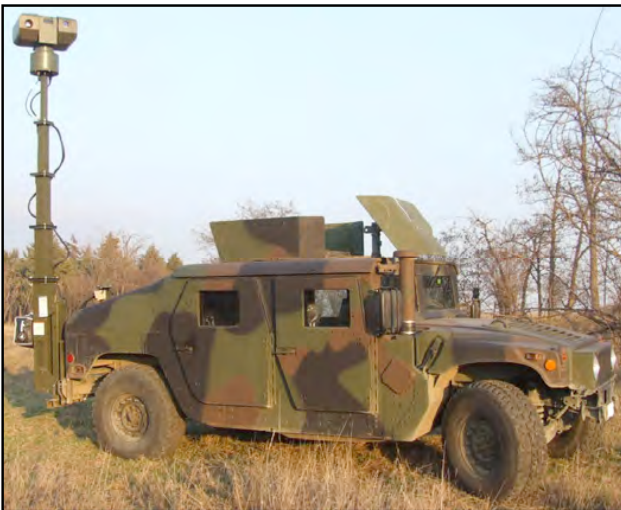
Fig. 69. A telescoping mast, with surveillance equipment on top, is mounted to the bumper of a humvee.
