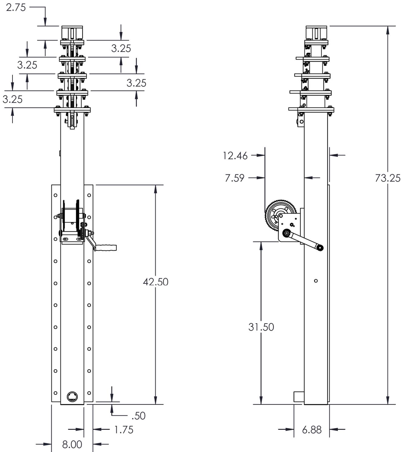
**Fig. 73.** A schematic of the EM25 mast showing it in the collapsed (stowed) configuration, which has an overall height of a little more than 6 ft, from two different angles. The small pipe pointing to the left and protruding from the bottom of the lowest stage associated with the telescoping mast unit (right schematic) is for pumping hot air into the mast in the event it gets frozen into place as a result of very cold and wet conditions. All dimensions are given in inches.
