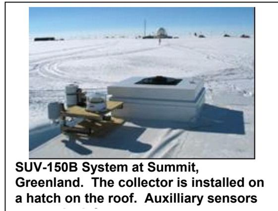
**SUV-150B System at Summit, Greenland. The collector is installed on a hatch on the roof. Auxilliary sensors**
