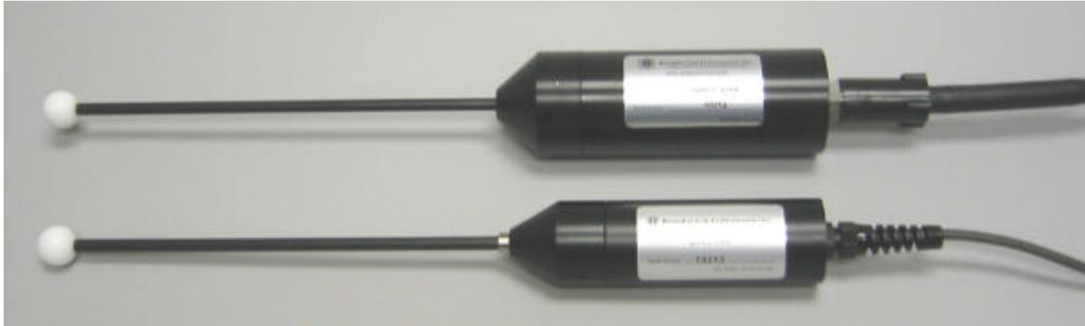
The QSL-2100 quantum scalar sensor features a 1.9 cm diameter Teflon® spherical optical collector and is designed to provide accurate measurement of photosynthetically active irradiance (PAR) in aquatic or dry environments. The small size of the scalar collector and convenient hand wand ensure that Biospherical Instruments' QSL sensors provide accurate light measurements from virtually all directions.
