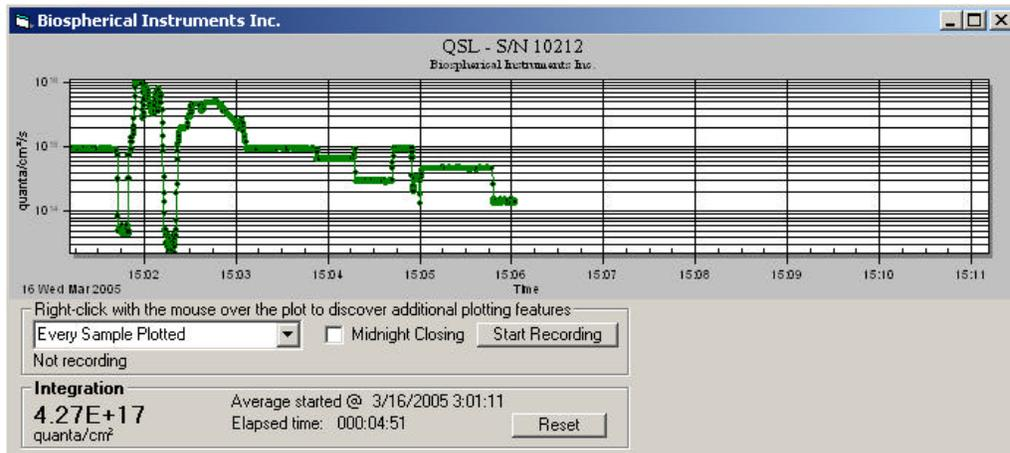
**Software:** LOGGER-2100 software is included with each sensor and is compatible with Windows 7, VISTA and XP. Data are in PC compatible digital format. The user may configure output for display in Quanta or Microeinstains.
