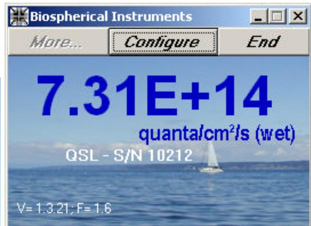
BSI's LOGGER-2100 software displays calibrated data in either Quanta or  $\mu$ Einsteins
