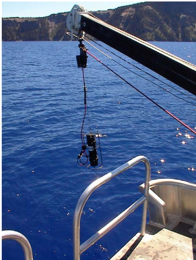
Supported by the telemetry cable, the PUV-2500 may be deployed by hand or using a winch
