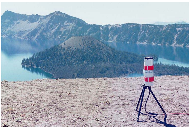
Supported by the telemetry cable, the PUV-2500 may be deployed by hand or using a winch
